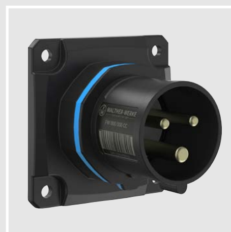
CEE NEO panel mount appliance inlet, straight, 3 x 16 A | 6 h | IP54 screw terminal or cage clamp connection
